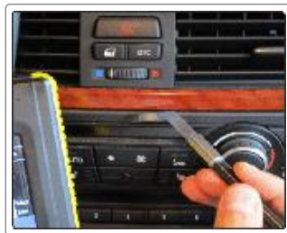
Measuring gaps on the car dashboard
