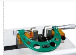
zero setting and calibration of micrometers
