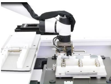
The robot automatically places the workpiece into OK or NG positions on the servo stacking&unloading
